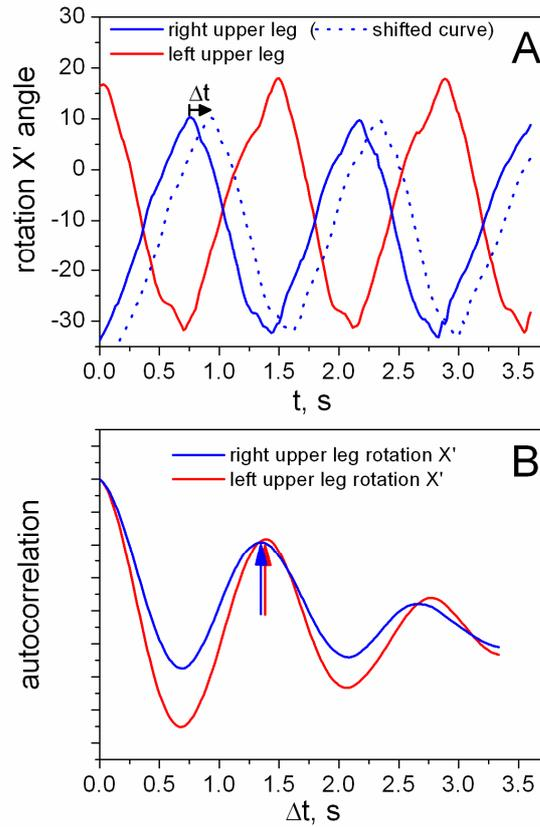
*Figure 4.* Examples of the angular data and computed autocorrelation curves. In panel A examples of actual sensor data for the upper leg sensors (continuous lines) as well as a shifted curve (dotted line). The autocorrelation functions (panel B) peak at the time-shift values where the shifted curve follows the original curve.
