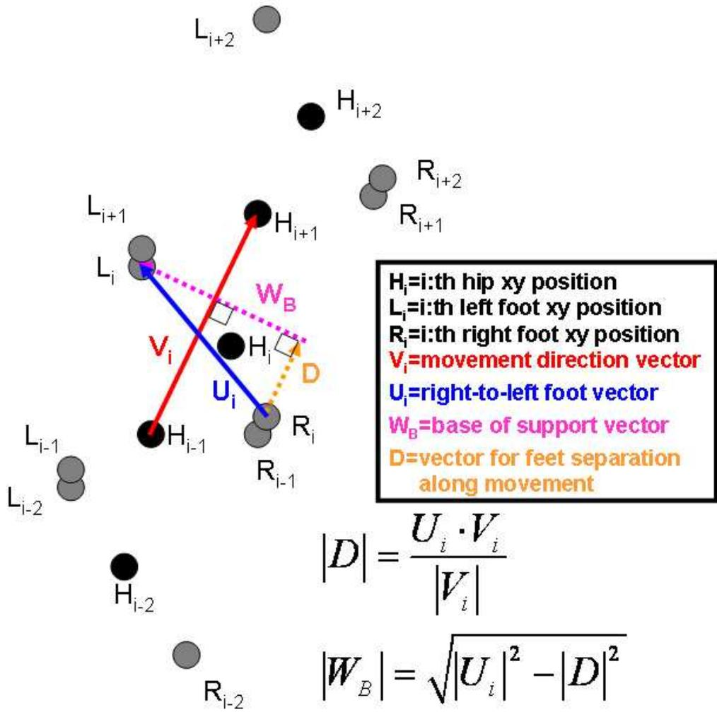
Figure 5. The calculation of the width for the base of support. The width for the base of support was calculated as the average of instantaneous values. At each time point  $i$  the instantaneous base width at a straight angle against the instantaneous direction of the movement was computed as shown in the figure.
